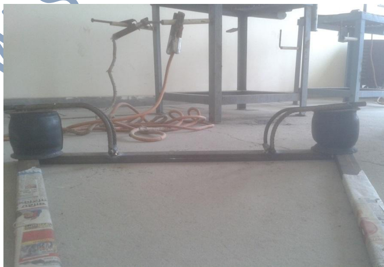
Fig. 5.2.3 (A-arm used for front suspension)
