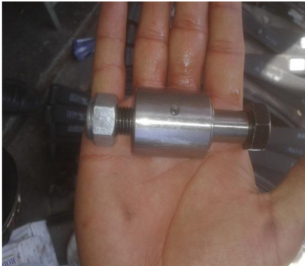
Fig.5.2.1 (Bush & rod assembly used for front wheels) Fig.5.2.2 (Bush & rod assembly used for rear wheel)
