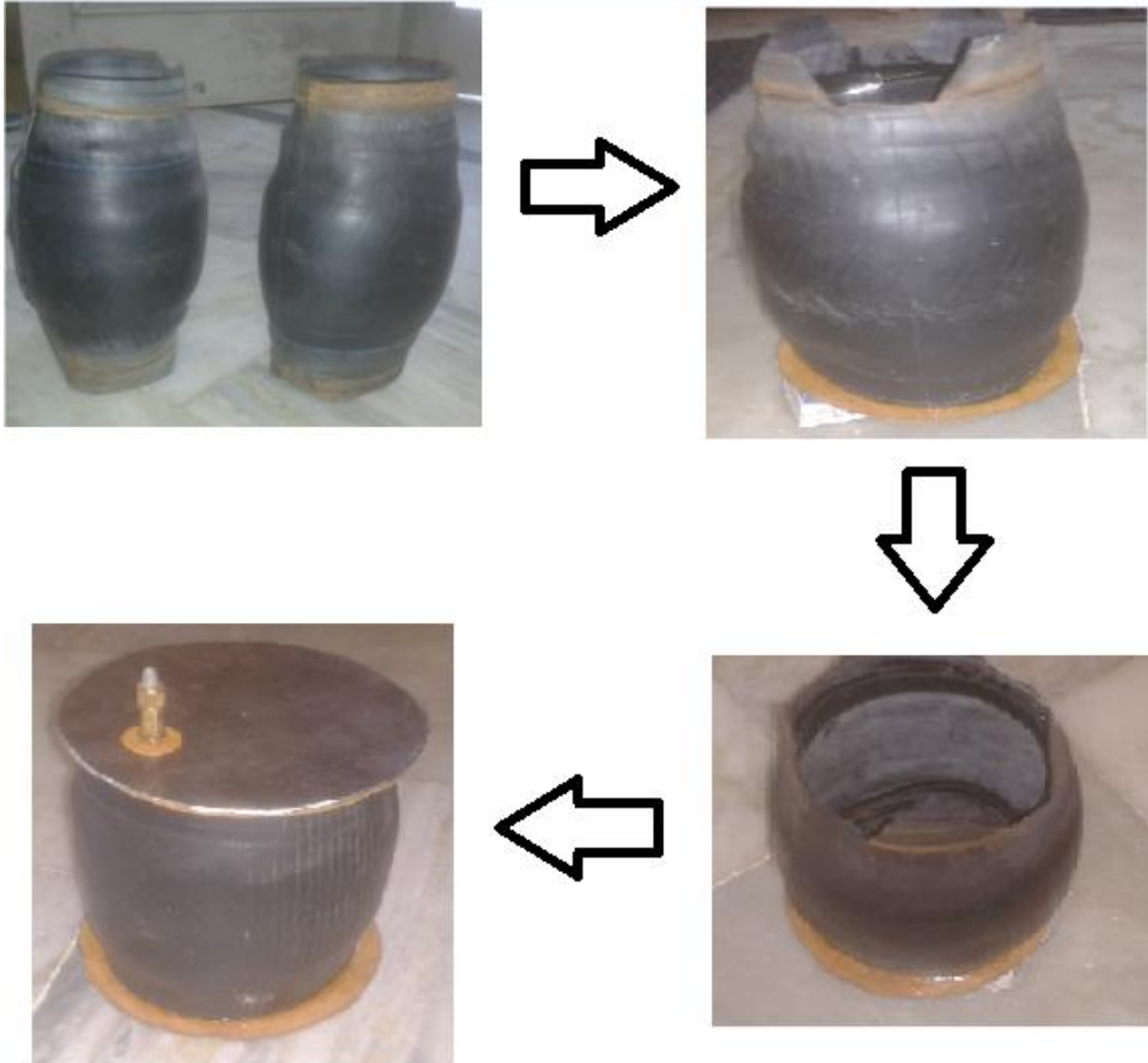
Fig.5.3.4 Steps of making of Air Bellow
