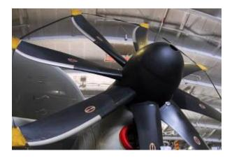
Photo: A turboprop engine uses a jet engine to power a propeller. Photo by Eduardo Zaragoza courtesy of US Navy.
