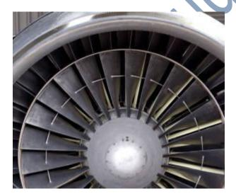
Photo: A turbofan engine produces more thrust using an inner fan and an outer bypass (the smaller ring you can see between the inner fan and the outer case). Each one of these engines produces 43,000 pounds of thrust (almost 4.5 times more than the Stratofortress engines up above)! Photo by Lance Cheung courtesy of US Air Force.
