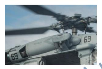
Photo: The gray tube you can see under the rotor of this US military Seahawk helicopter is one of its twin turboshaft engines. There's another one exactly the same on the other side. Photo by Trevor Kohlrus courtesy of US Navy.
