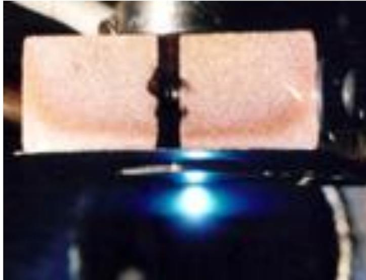
This source of extreme ultraviolet light is based on a plasma created when a laser is focused on a beam of xenon gas clusters expanding at supersonic speeds. (Besides invisible-to-the-eye extreme ultraviolet light, some visible light is also created, as seen in the blue glow in the photo.)
