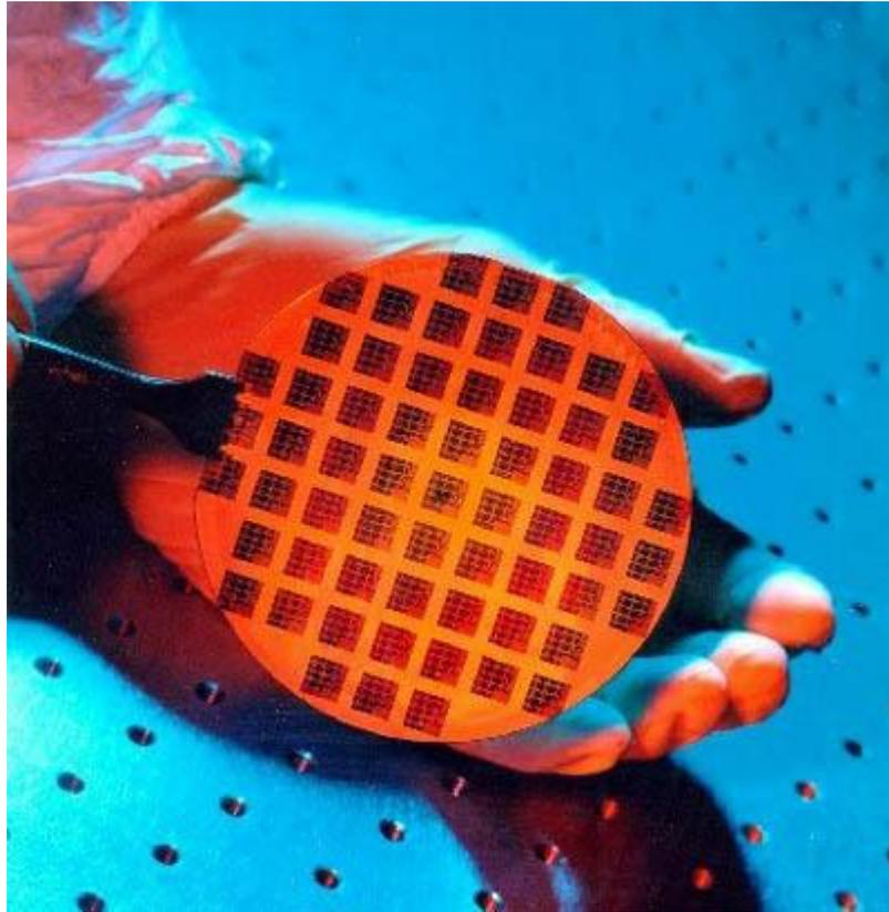
This wafer was patterned on a prototype device using extreme-ultraviolet lithography (EUVL).
