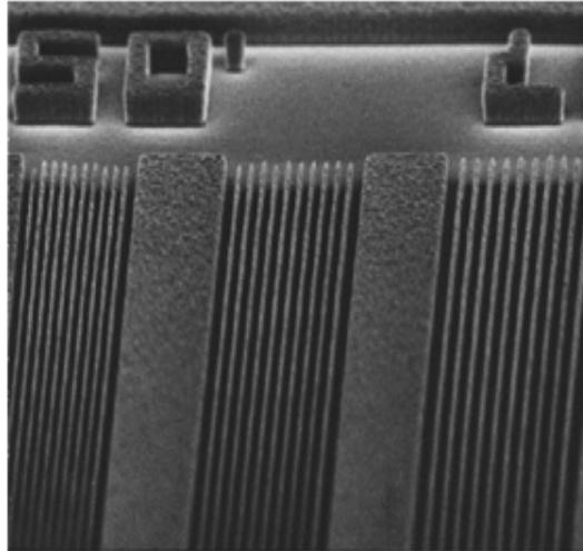
Using a prototype system, the Virtual National Laboratory has successfully printed lines as small as 50 nanometers (billionths of a meter) wide in photoresist. Current lithographic tools used in the semiconductor industry print patterns with 180-nanometer-size features.
