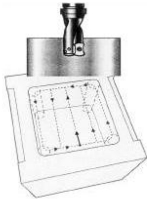
Fig. 5. Example of machining a cavity with predrill a starting hole [2].
