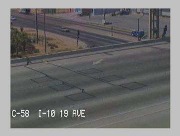
Notice the loop detectors placed in the road. As cars pass over the loops, the detectors are able to detect speed and movement.
