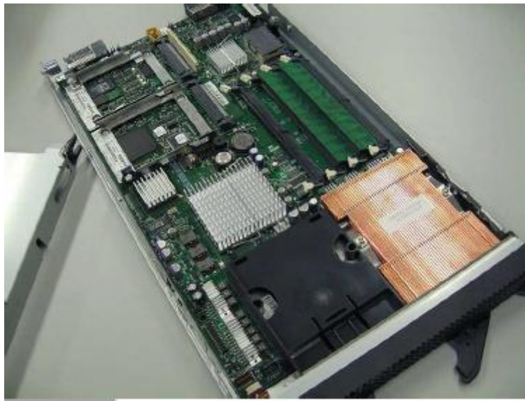
IBM HS20 blade server. Two bays for 2.5" (6.4 cm) SCSI hard drives appear in the upper left area of the image
