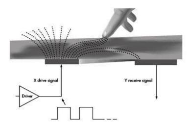
The projective screen contains a sensor at every intersection of the row and column, thereby increasing the accuracy of the system. There are two types of projected capacitive touchscreen: Mutual Capacitance and Self Capacitance.
