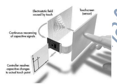
In the Projected-Capacitive Touchscreen Technology, the conductive ITO layer is etched to form a grid of multiple horizontal and vertical electrodes. It involves sensing along both the X and Y axis using clearly etched ITO pattern.
