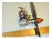
An idea of the size of the *Nano* is given by this picture. From backplate to drive washer is less than 1 inch. There are no exotic materials required. The crankcase is hacked from a solid cube of aluminium 3/4" on a side. The piston and contra piston are cast iron. The crankshaft and liner are any old steel from the scrap box.
