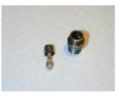
The cutter is used to form the exhaust ports in the cylinder. There are three of these, spaced at 120 degrees with sufficient space between them for the angled transfer ports to slightly overlap the timing. The crown of the piston is conical to assist transfer. The contra piston has a matching concave conical depression.
