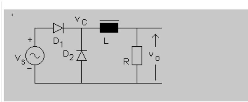
The circuit shown above differs from the circuit described in the previous page, which had only one diode, labeled  $D_1$ . This circuit has another diode, marked  $D_2$  in the circuit shown above. This diode is called the free-wheeling diode. The circuit operation is described next. The explanation is based on the assumption that the reader knows how the circuit without a free-wheeling diode operates.
