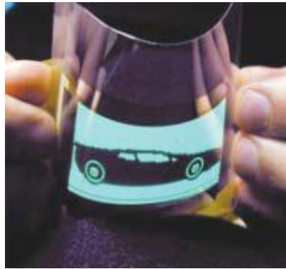
A PASSIVE-MATRIX 0.18MM THICK FOLED FABRICATED IN UDC'S PILOT LINE FACILITY
