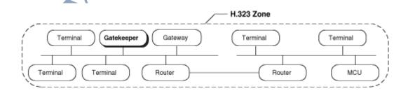
Gatekeepers perform two important call control functions. The first is address translation from LAN aliases for terminals and gateways to IP or IPX addresses, as defined in the RAS specification. The second function is bandwidth management, which is also
