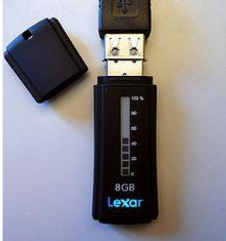
USB flash drive with E Ink-implemented capacity meter of available flash memory
