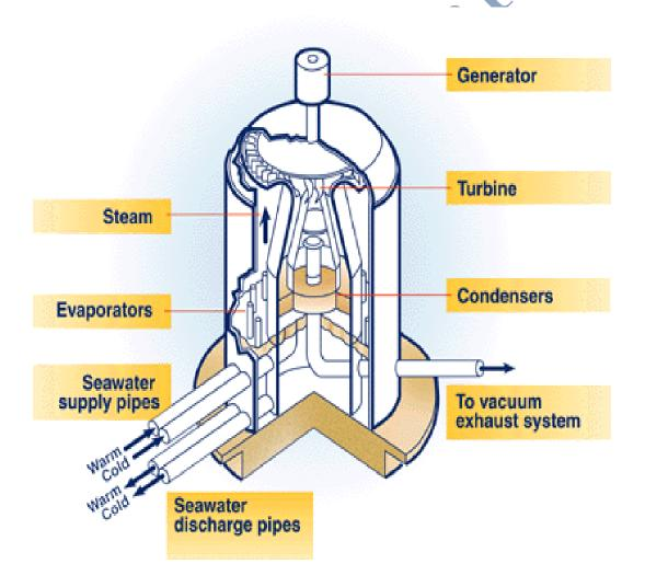
In May 1993, an open-cycle OTEC plant at Keahole Point, Hawaii, produced 50,000 watts of electricity during a net power-producing experiment. This broke the record of 40,000 watts set by a Japanese system in 1982. Today, scientists are developing new, cost-effective, state-of-the-art turbines for open-cycle OTEC systems.
