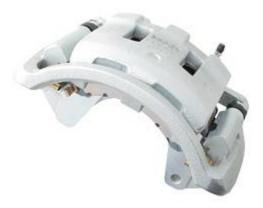
Disc brakes are used mainly in passenger cars, but due to their stable performance at higher speeds and resistance to brake fade, they are gradually spreading into the commercial vehicle segment, where drum brakes were traditionally chosen for their long lining life.
