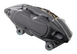
This type of disc brake has pistons on both sides of the brake rotor, and there are no moving parts in the caliper assembly other than the pistons themselves. This type of caliper provides very even pressure distribution between pads and rotor providing better braking performance, especially under severe braking conditions.
