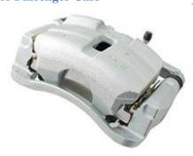
Floating caliper type disc brakes have a piston (or pistons) only on the inner side of the rotor. When the brake is engaged, a piston pushes the inner brake pad against the rotor. This generates a reaction force that moves the caliper itself along the slide pin, pushing the outer pad against the rotor to clamp it from both sides and achieve braking action.
