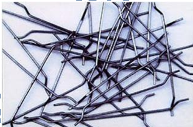
Fig.3.1 Shape of steel fibres (properties of PSFC, Li, Zhao).
