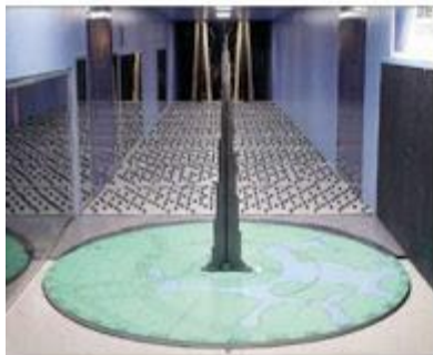
Figure 11. Aeroelastic wind tunnel model
