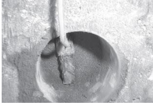
Fig. 2.8 Use of rebar probes in instrumentation
