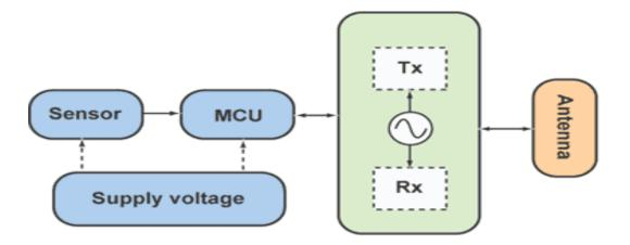
3. This diagram shows a wireless sensor node architecture.
