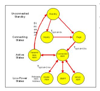
The communication protocol is described by the following state diagram. Standby is the default state.
