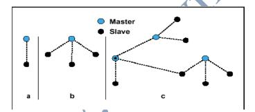
**SCATTERNETS:** Two or more piconets with overlapping coverage areas form the scatternet. Slaves in one piconet can be master or slave in the other piconet [Achieved by TDM]. Up to 10 fully loaded piconets can coexist in a scatternet. Any devices in multiple piconets employ TDM. The two types of links that can be establishes between the master and slaves are named
