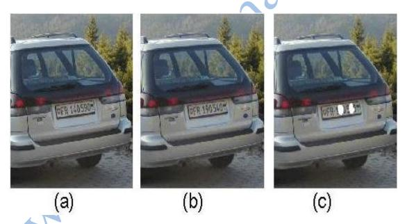
Using digital watermarks for integrity verification: the protected image is the image (a) above; a modified image is obtained by swapping the numbers 9 and 4 of the number plate (b); digital watermarking technology allows detecting and highlights the modified areas, as shown on (c).
