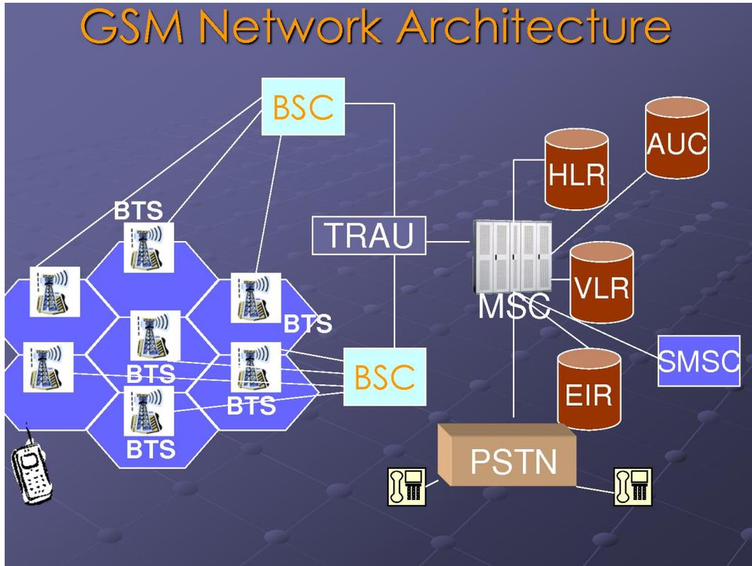
The MS and the BSS communicate across the Um interface, also known as the air interface or radio link. The BSS communicates with the Network Service Switching center across the A interface.
