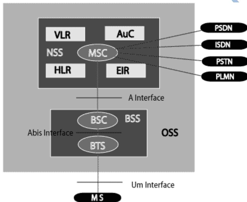
The added components of the GSM architecture include the functions of the databases and messaging systems:
