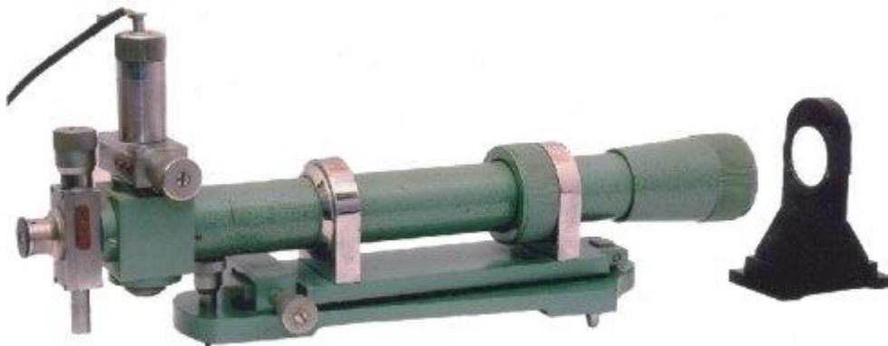
If the reflector is tilted through a small angle ( $\theta$ ) the parallel beam will be reflected through twice the angle ( $2\theta$ ) and would be brought to focus in the same plane as the light source but to one side of it. The image will not coincide but there will be a distance equal to focal length times the angle of reflection ( $2f\theta$ ) where  $f$  is the focal length of the collimating lens.
